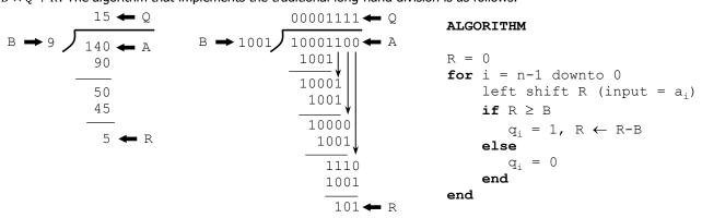
• An iterative architecture is depicted in the figure for *A* with 6 bits and *B* with 4 bits. The register *R* stores the remainder. A division operation is started when *E* = 1 (where *A* and *B* values are captured). Then, at every clock cycle, we either: i) shift in the next bit of *A*, or ii) shift in the next bit of *A* and subtract *B*. The signal *done* is asserted to indicate that the operation has been completed and the result appears in *Q* and *R*.
